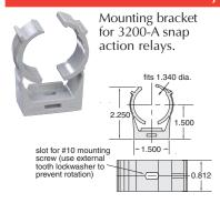
Part No. 3200-006 Snap Action Relay Bracket
